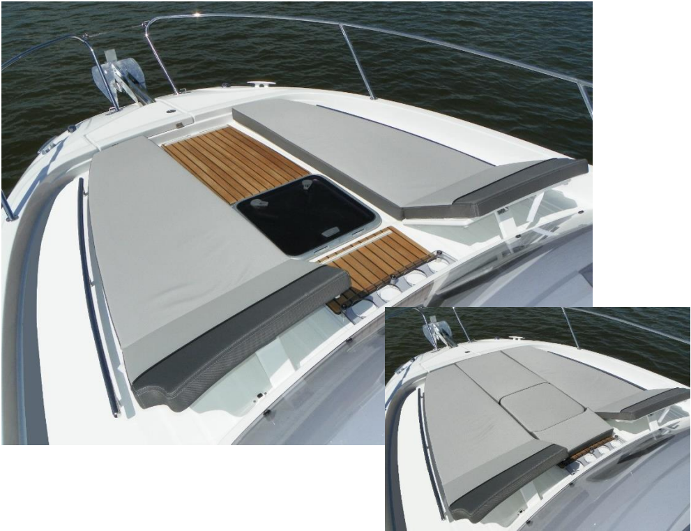
Front sundeck with lifting backrests + handrails : easy access at the anchor locker without to remove cushions
