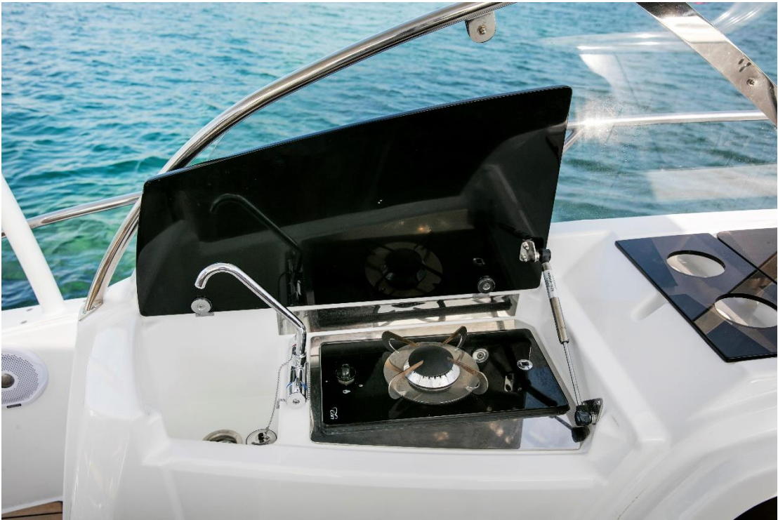
Cockpit galley with sink (standard) and gas burner (option)
