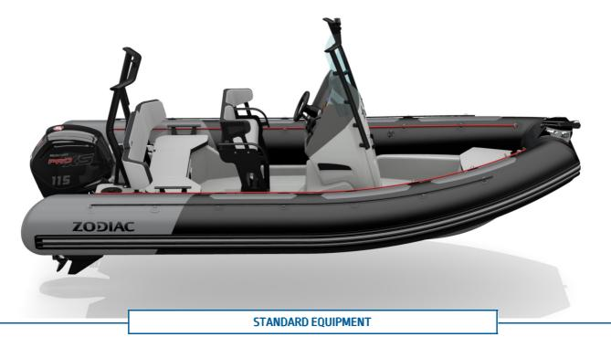
HULL & DECK: 1 Bow Bitt/2 Aft Cleats, 1 Bow D Ring/2 Towing Rings, 2 Bailers, Built-in Fuel Tank 100L, Fairleads, GRP Deep V-Hull, Lockable Mooring Storage, Ski & Wakeboard Locker, Tilting Console.
